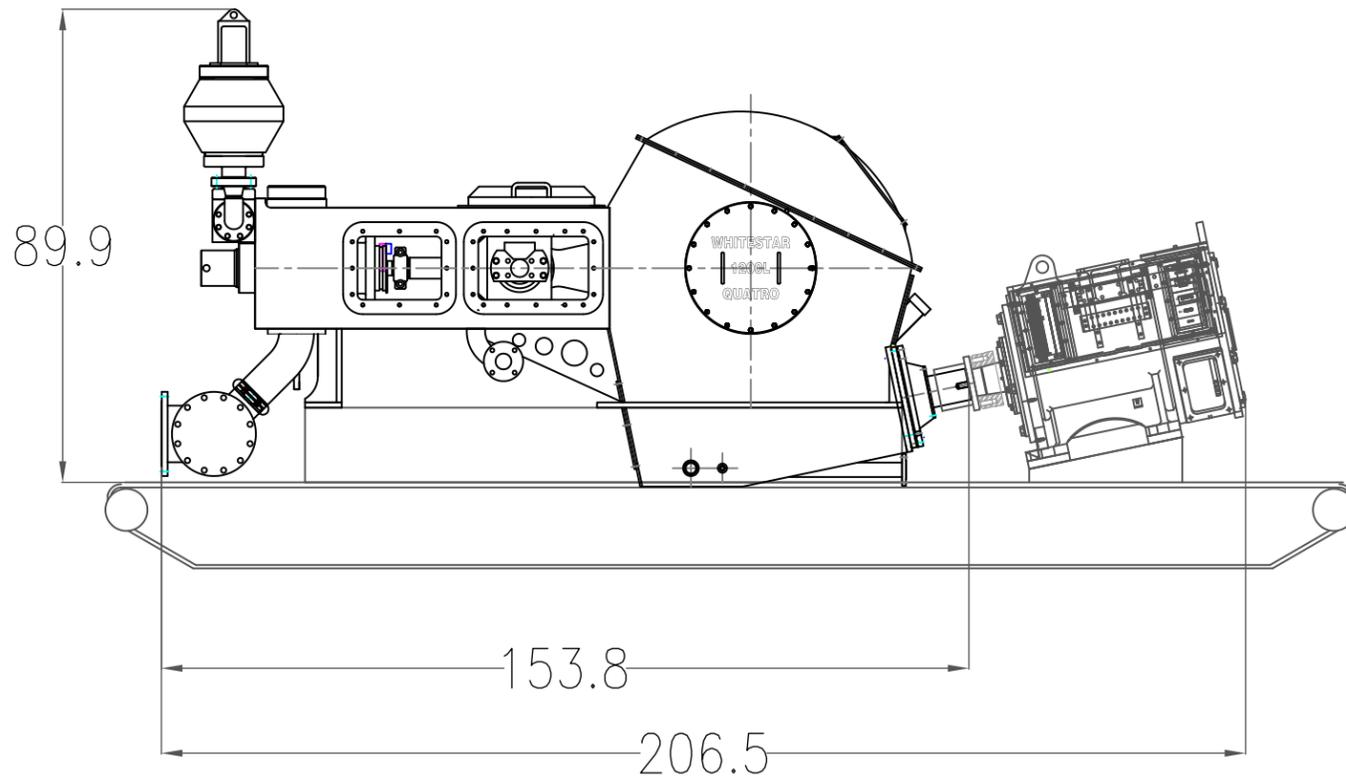
OVERALL DIMENSIONS OF PUMP & ENGINE: 207 " L X 64" W X 89.9" H
