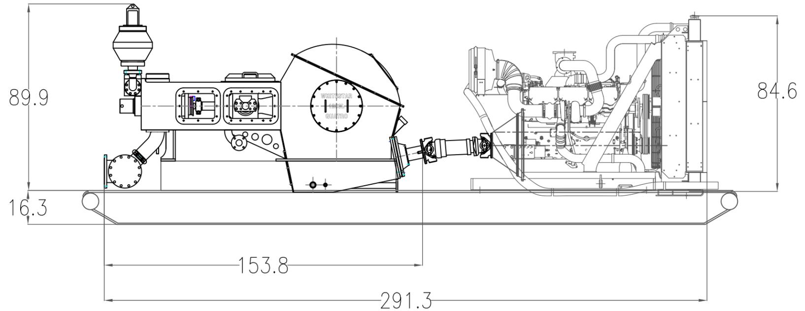
OVERALL DIMENSIONS OF PUMP & ENGINE: 292 " L X 64" W X 89.9" H
