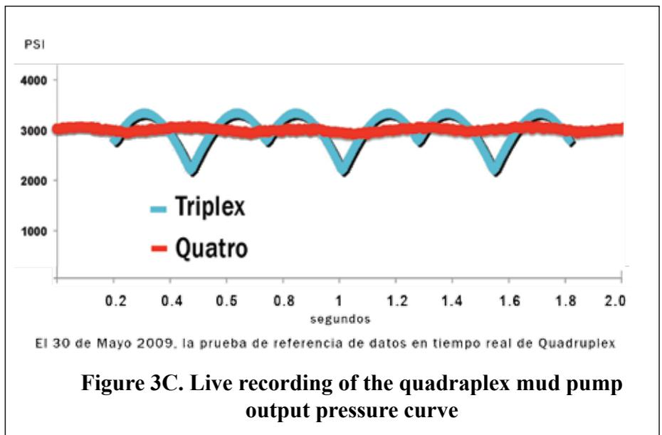
drill system pressure changes due to the added surge down the drill string and through the down hole tools and drill bit. The resulting pressure change is much greater than the flow rate change.
