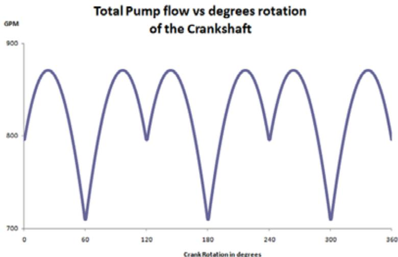
However, the maximum flow in the cylinder at the peak speed of 380 fpm is 871 gpm, more than three times the cylinder average flow rate.
